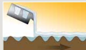
The two-layer curtain coating covers the brown base and increases brightness.
